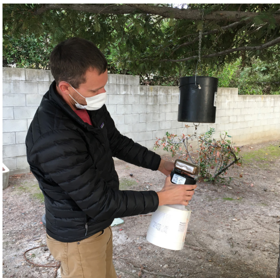
District Vector Ecologist Eric Ghilarducci prepares a trap to capture adult mosquitoes by using dry ice to simulate human breath to attract the mosquitoes.
