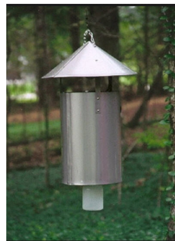
A New Jersey light trap hangs ready to trap adult mosquitoes. A 2-watt LED bulb attracts night-flying mosquitoes.
