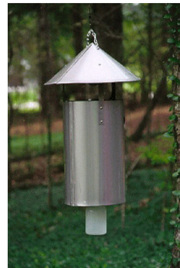
A New Jersey Mosquito light trap used to collect adult mosquitoes.
