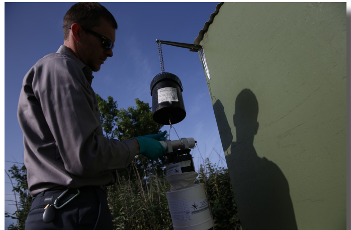
District Vector Ecologist Eric Ghilarducci prepares a trap to capture adult mosquitoes by using dry ice to simulate human breath to attract the mosquitoes.
