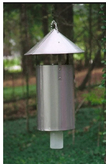
A New Jersey light trap hangs ready to trap adult mosquitoes. A 5-watt fluorescent bulb attracts night-flying mosquitoes.
