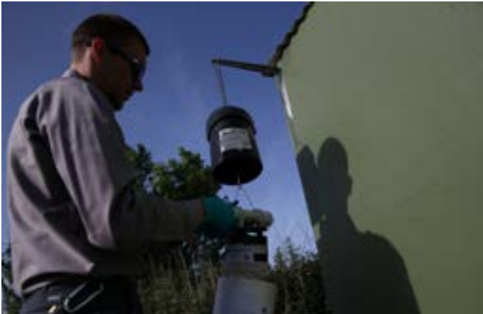
District Vector Ecologist II Eric Ghilarducci prepares a trap to capture adult mosquitoes.
