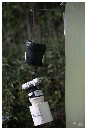
A CO 2 trap hangs ready to trap adult mosquitoes. Dry ice produces carbon dioxide, which simulates the breath of a person and attracts adult mosquitoes.
