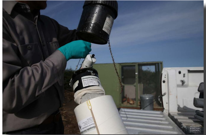
District Ecologist Eric Ghilarducci prepares a trap to capture adult mosquitoes. The trap uses dry ice as bait to trap the mosquitoes, simulating the breath of a person.
