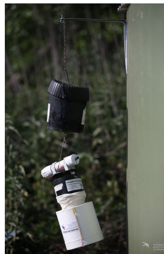
A CO 2 trap hangs ready to trap adult mosquitoes. Dry ice produces carbon dioxide, which simulates the breath of a person or animal and attracts adult mosquitoes.
